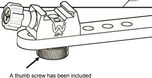
A thumb screw has been included to allow tool free installation in the field for this application.
